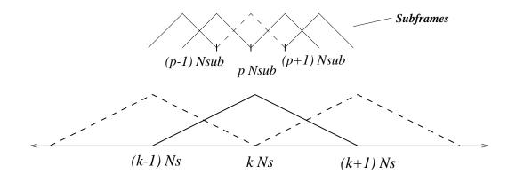
Figure 2: Subframe overlap-add synthesis.
